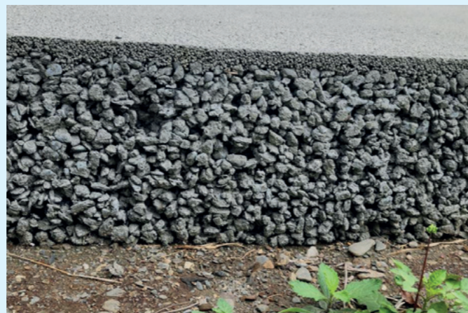
Top: TCC DAKA Renewable Resource Recycling Centre Above: Permeable concrete used for roads can withstand 210kg per cm 2 pressure, meeting strength, carbon reduction, and environmental protection standards
