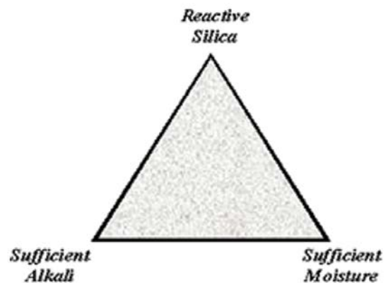
Figure 4.14: Essential factors for propagation of ASR [76]
